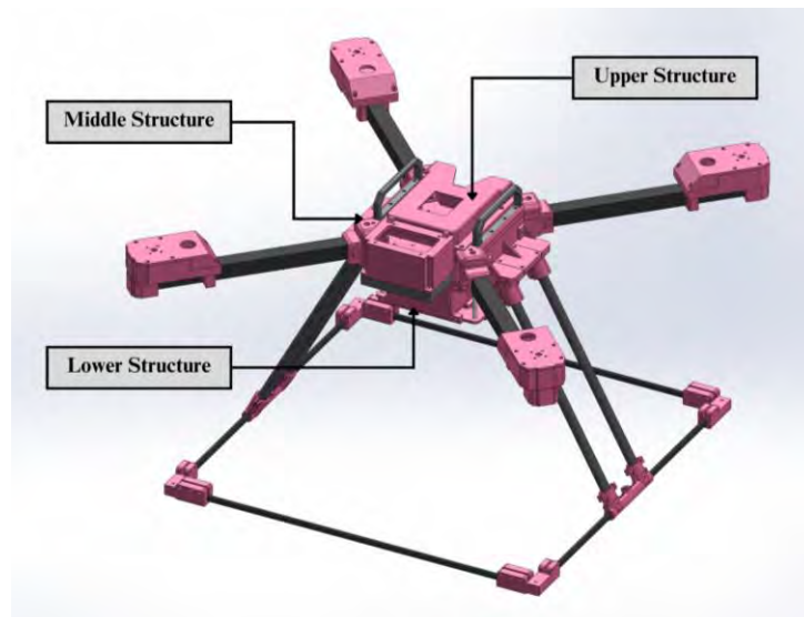
Figure 1: Design of the semi-autonomous UAV structure
