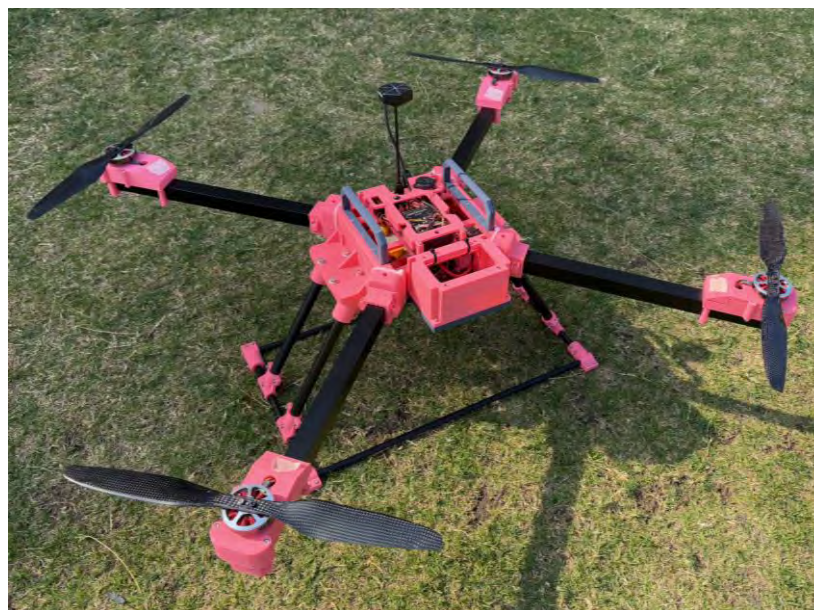
Figure 6: Prototype semi-autonomous UAV for emergency medical supply delivery in disaster-affected and hard-to-reach areas
