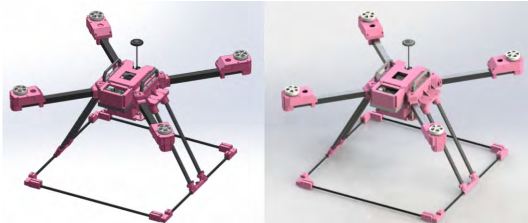
Figure 3: Design of the semi-autonomous UAV for emergency medical supply delivery in disaster-affected and hard-to-reach areas
